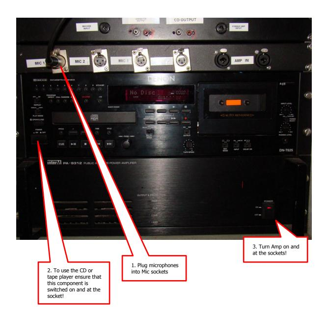
b. In the cupboard (back left of hall) ensure that the cables are connected correctly. Line 1-4 plugs have labels on the cables and must be correctly connected. If using the CD player ensure that the red and white plugs are connected to the CD socket (likewise for the tape deck). The two black leads must be connected to the Main Amp Input plugs.
